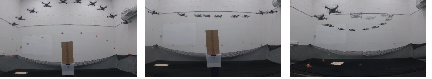
(a) Obstacle avoidance without waypoint guidance (b) Obstacle avoidance with lateral waypoint guidance (c) Payload waypoint navigation with horizontal waypoint guidance
