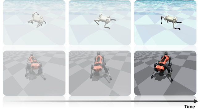
Fig. 8: Robot Walking Visualization. Top: A1 robot is prompted to walk on uneven terrain in MuJoCo, where the LLM policy can make it recover from terrain disturbance. Bottom: ANYmal robot is prompted to walk on flat ground in Isaac Gym using the same approach.
