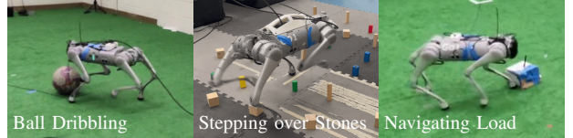
Fig. 1: The proposed HiLMA-Res framework enables a quadrupedal robot to perform different loco-manipulation tasks in the real world. These include dribbling a ball in a desired direction, stepping over small blocks scattered on the ground, and navigating a load to the desired goal through real-world learning. We highlight the versatility of the HiLMA-Res framework in various loco-manipulation tasks with different observation spaces and learning algorithms. We encourage readers to view the supplementary video at https://youtu.be/8dOs9_RDn4E for more results.
