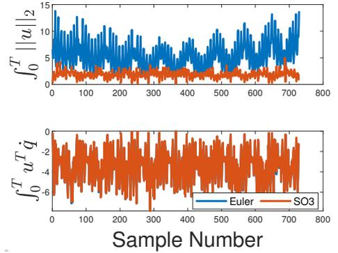
Fig. 7. The top plot shows normed input integral and the bottom plot shows power integral for each experiment. Note that *orange* points indicate  $\tilde{u}_e$  and *blue* points indicate  $u_e$ .
