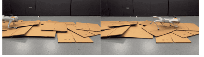
(a) Snapshots of the quadruped robot climbing over randomly distributed paper boards.
