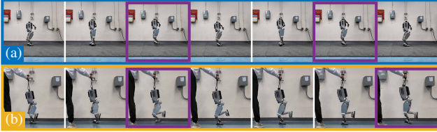
Fig. 7. Hopping with (a) both legs and (b) a single leg, with noticeable flight phases marked with purple frames.
