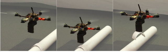
Fig. 10. Still images from a sample “swooping” trajectory using the vision-based controller developed in this paper. The background has been washed out slightly to improve visibility.
