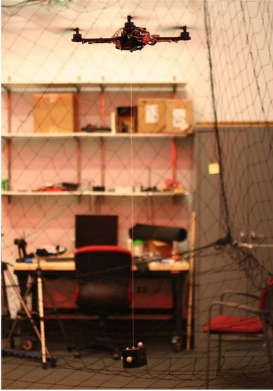
Fig. 5: A Hummingbird quadrotor with a cable suspended load. Both the quadrotor and the suspended load are equipped with Vicon markers for enabling sensing their position and attitude for feedback control. The cable length is 1 m, and the load weighs 90 gm.
