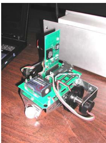
Fig 5: Inexpensive Rover Unit for color-based indoor adaptive sampling algorithm validation testbed.
