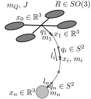
Fig. 2: Quadrotor with a point-mass payload suspended through a flexible cable. The flexible cable is modeled as a series of links connected by  $S^2$  joints. The system evolves on  $SO(3) \times \mathbb{R}^3 \times (S^2)^n$  and has  $(6 + 2n)$  degrees of freedom with  $(2 + 2n)$  degrees of underactuation.
