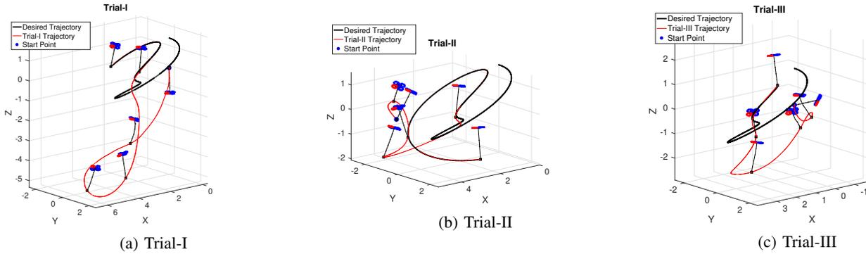
Fig. 4: Snapshots of quadrotor with load suspended by flexible cable at various instances of time along the trajectory (red) obtained through variation based linearization controller to track the reference trajectory (black).
