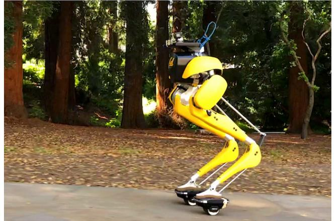
Fig. 1: Snapshot of an experiment of the bipedal robot Cassie autonomously riding on Hovershoes. Experimental videos are at [https://youtu.be/b2fKBb\\_0iTo](https://youtu.be/b2fKBb_0iTo).
