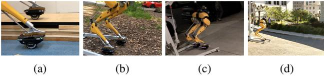
Fig. 9: Cassie riding the Hovershoes on (a) different heights, (b) rough terrain, (c) up a  $7^\circ$  incline, and (d) down a  $13^\circ$  incline.
