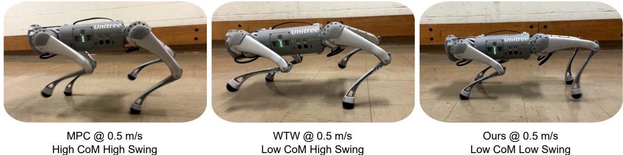
Fig. 5: Three policies walking at 0.5 m/s. Built-in MPC and walk-these-ways (WTW) [3] swing the legs to a redundant height, while our policy only makes necessary lifting of the leg. This demonstrates the energy-efficiency of our policy.
