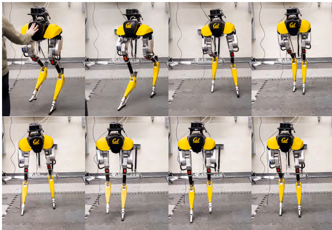
Figure 4.6: Snapshots of Cassie robot illustrating recovery from a push in the backwards direction. The first and the last tiles are about 3s apart.
