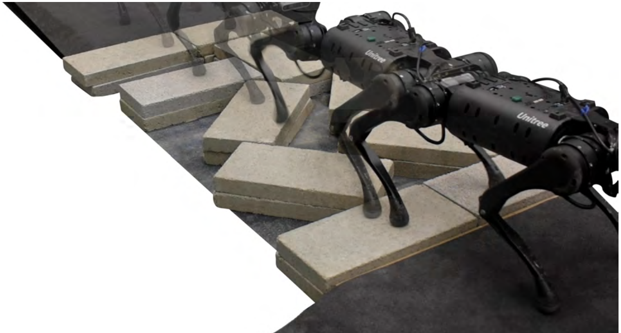
Figure 5.1: The A1 quadruped robot walking over a random discrete terrain using our proposed approach.
