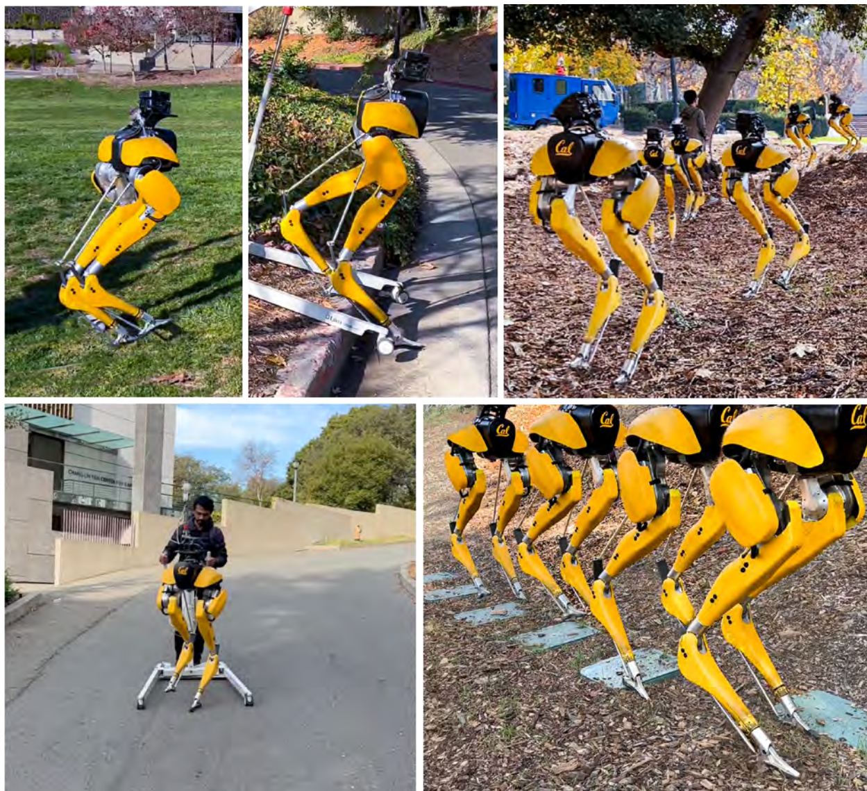
Figure 4.12: Snapshots of outdoor walking experiments. Using the proposed approach, Cassie is able to negotiate a wide variety of terrain, including paved concrete roads and sidewalks, grass, and loose soft ground such as mulch. Cassie is also able to tackle large sloped terrains (uphill and downhill), as well as step across curbs. Note that in all experiments, Cassie is blind and cannot perceive the surrounding terrain.
