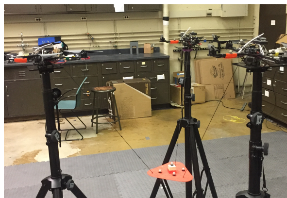
(b) Experimental setup of rigid-body load.
