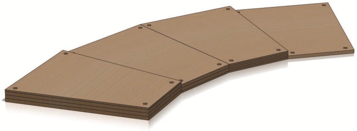
Figure 25: Plywood boards used to form a stair-stepped platform. By combining boards that are 1 inch (2.54 cm) and 0.5 inch (1.27 cm) thick, platforms of a desired height are assembled.
