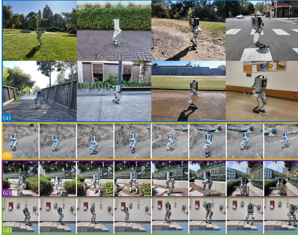
Figure 5: Walking on Various Terrains. (a) The robot walks on eight different types of terrain. (b) The robot climbs a relatively steep and narrow unpaved trail covered with dust and rocks. (c) The robot walks on an uneven pathway. (d) The robot makes a turn on rocky stairs.
