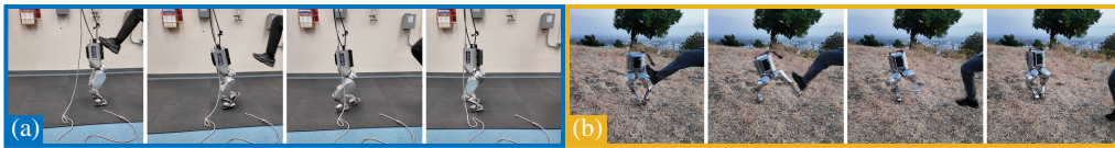
Figure 6: Disturbance Rejection. The robot is able to recover from large external perturbations, such as being kicked (a) from behind while walking in the lab, and (b) from the side while walking in the wild.
