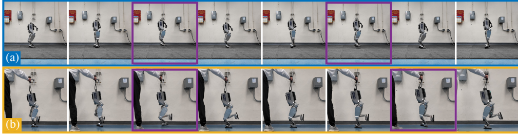
Figure 9: Hopping with (a) both legs and (b) a single leg, with noticeable flight phases. Being able to accomplish dynamic tasks with a simple RL controller shows the small sim-to-real gap of the hardware design. The purple frames indicate that the robot is in the flight phase.
