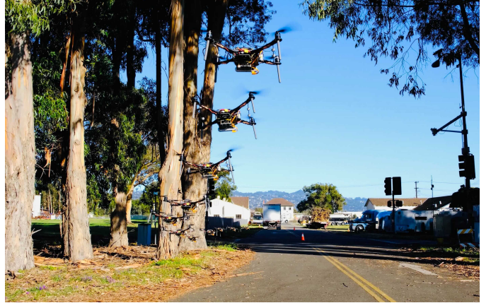
Figure 1. The perception-aware planner guides the quadcopter to fly close to areas with more visual features for better VIO accuracy – the paved road has much fewer visual features than the trees. The goal is 20 meters forward from the starting position of the vehicle, which is in the direction away from the camera taking this photo.
