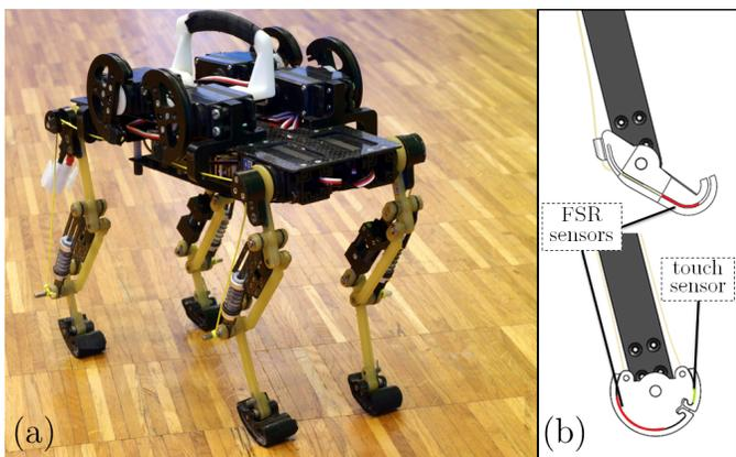
Fig. 1. a) Cheetah-Cub robot. b) Two examples of foot designs: *top*, spring-loaded foot with compliant sole and force sensor; *bottom*, ball-foot equipped with ground force sensor and stumble detector.
