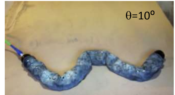
Slipping failure ( I/L=1 )
