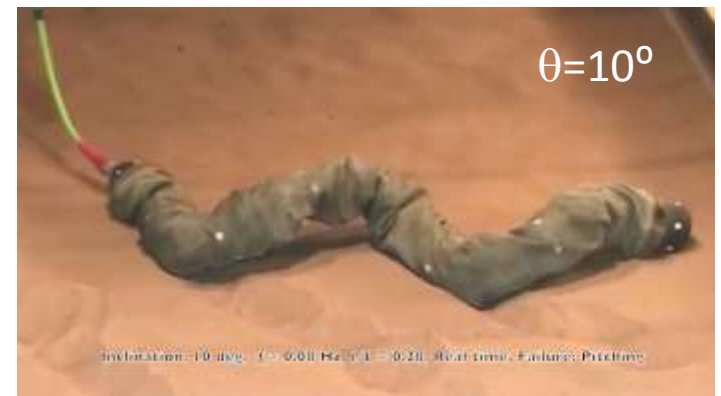
Pitching failure ( I/L=0.27 )
